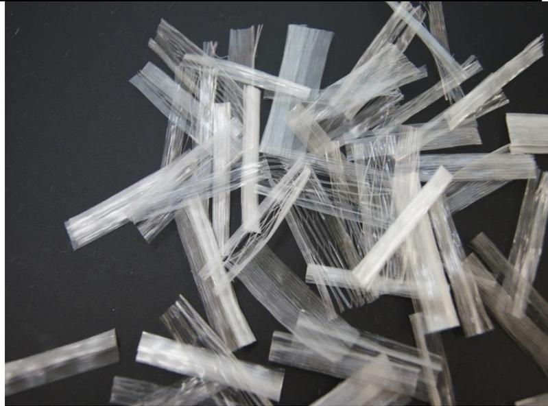
**Guidelines for use:** The recommended dosage for **F-Macro** fiber is 3 lbs. per cubic yard. **F-Macro** can be used at a dosage rate of up to 10 lbs. per cubic yard. For composite metal deck applications, minimum dosage rate is 4 lbs. per cubic yard as recommended by the Steel Deck Institute.
