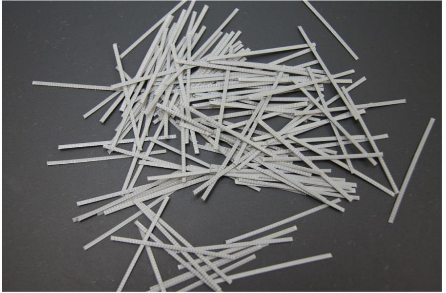
**Guidelines for use:** The recommended dosage for **M-Macro** fiber is 3 lbs. per cubic yard. **M-Macro** can be used at a dosage rate of up to 10 lbs. per cubic yard. For composite metal deck applications, minimum dosage rate is 4 lbs. per cubic yard as recommended by the Steel Deck Institute.
